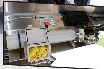
In the event of an emergency due to electrical or mechanical issues the EZ Flow<sup>XR</sup> doors can be easily converted into manual operation. The emergency manual override utilizes quick release pins and straps to open the door. This new override system is not only easy to use, but provides additional ground clearance compared to previous override systems.
