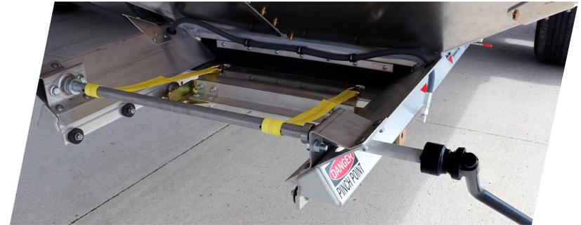
In the event of an emergency due to electrical or mechanical failures the EZ Flow<sup>XR</sup> doors can be easily converted into manual operation. The emergency manual override utilizes quick release pins and straps to open the door. This new override system is not only easy to use, but provides additional ground clearance compared to previous override systems.
