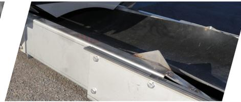
Conveyor is constructed of high quality 304 stainless steel
