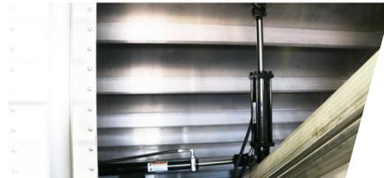
The vertical hydraulic cylinders move the upper conveyor tube up and down while the horizontal hydraulic cylinder moves the conveyor tube left to right by 9 degrees.
