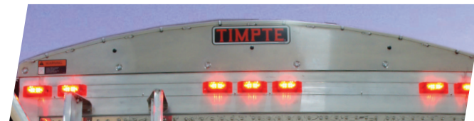
7 LED Lights on Rear Header 4 Outside Lights Turn/Clearance 3 Inside Lights Stop/Clearance
